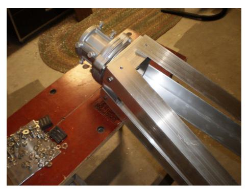
6. Tilt the assembled structure upright and spread the legs apart by about 27 inches (similar to unfolding a step ladder). Assemble the cross braces, upper shelf bracket and lower shelf bracket (with rotor shelf mounting holes) on each of the 2 open sides as shown below, using  $\frac{1}{4}$  20 x 1" bolts, lock-washers and nuts. Hand-tighten the hardware at this time.
