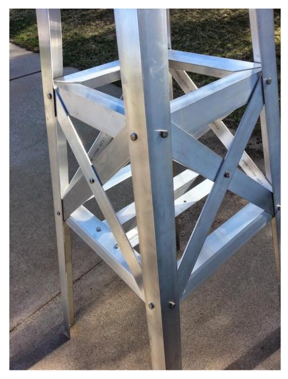
7. Attach the 2 rotor shelves to 2 of the lower shelf brackets with 4 each  $\frac{1}{2}$ "-20 x 1" bolts, lock-washers and nuts as shown below. Verify that all rotor mounting holes are 3.31" (Yaesu) or 3.0" (Hy-Gain) or 2.5" (MC-10) apart, then tighten these bolts securely.
