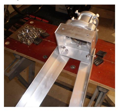
5. Assemble a second leg assembly identical to the one assembled in Step 3. Lay this assembly on top of the first leg assembly. The feet attachment holes should be facing up. Attach to the top assembly as shown below. Use 4 each  $\frac{1}{2}$  20 x 3/4" bolts, lock-washers and nuts. Hand-tighten the hardware at this time.
