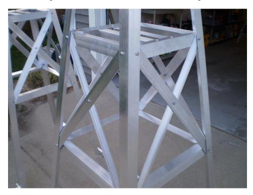
7. Attach the 2 rotor shelves to 2 of the upper shelf brackets with 4 each  $\frac{1}{2}$ "-20 x 1" bolts, lock-washers and nuts as shown below. Verify that all rotor mounting holes are 3.31" (Yaesu) or 3.0" (Hy-Gain) or 2.5" (MC-10) apart, then tighten these bolts securely.
