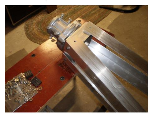
6. Tilt the assembled structure upright and spread the legs apart by about 32 inches (similar to unfolding a step ladder). Assemble the cross braces, upper shelf bracket (with rotor shelf mounting holes) and lower shelf bracket on each of the 2 open sides as shown below, using  $\frac{1}{4}$  20 x 1" bolts, lock-washers and nuts. Hand-tighten the hardware at this time.
