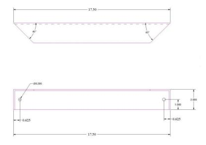
Lower Shelf (2), For the HD version, all drilled holes are 0.375" diameter.
