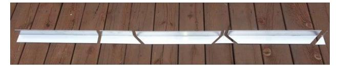
The 2" x 2" x **1/4"** x 24" long angle is cut into 4 equal length sections with straight cuts. These are the 4 tower Feet, <u>approximately</u> 6" in length.
