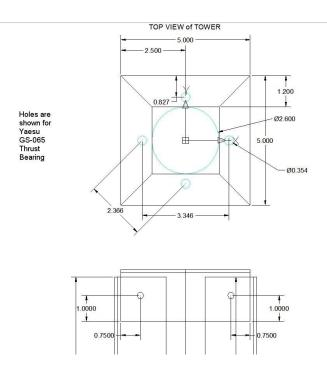
The four Lower Shelves are divided into two groups of two. Two shelves have holes drilled for attachment to the Legs and the Rotor Shelf. The two remaining Lower Shelves only have the holes drilled for attachment to the Legs. See the two drawings below. For the HD version, all drilled holes are 0.375" diameter.
