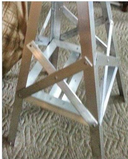
9. Attach the 2 rotor shelves to the lower shelf brackets with 4 each  $\frac{1}{4}$ "-20 x 1" bolts, lock-washers and nuts as shown above. Verify that all rotor mounting holes are 3.31" (Yaesu) or 3.0" (Hy-Gain) or 2.5" (MC-10) apart, then tighten these bolts securely. See the image at right above.
