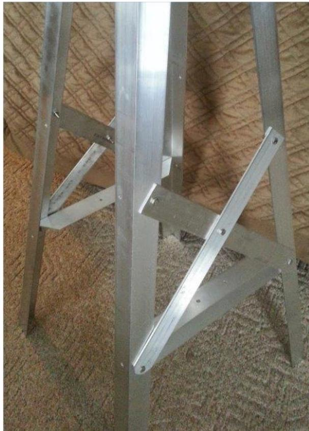
7. Attach the remaining 2 sets of X-braces on each of the 2 open sides as shown below, using  $\frac{1}{4}$ "-20 x 1" bolts, lock-washers and nuts. Spread the tower legs apart until the lower holes of the X-braces line up with the holes in the tower legs. Hand-tighten the upper set of bolts in these 2 assemblies at this time. See the image below.
